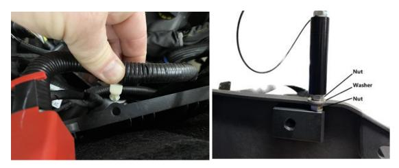
**B\* Optional Step.** To increase the stability of the mount, start by marking the location of the hole in the support block, drill a 3/8 hole (this is best done with the battery removed) and install a 3/8-24 bolt from the inside of the battery tray out through the bracket. You will need to cut a small portion of the inner support ribs to make room for the bolt.
