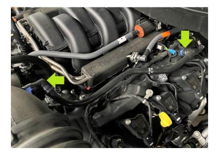
Install the CSS onto the Valve cover fitting by lifting up on the collar at the base, and then pushing down on the CSS. The collar will click when fully engaged. Connect the hose from the CSS to the air intake tube.
