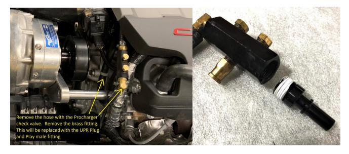
2. Locate the hose that runs from the lifter valley PCV fitting to the brass fitting on the Procharger vacuum block. This hose will have a check valve in it. Remove the hose, check valve and brass fitting from the vacuum block. The vacuum block will remain connected to the vacuum fitting on the intake manifold. Install the provided UPR 3/8NPT to Plug and Play™ fitting into the vacuum block.
