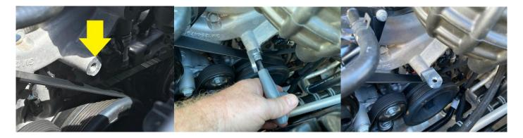
1. Locate the un-used bolt boss on the water pump housing just above the crank pulley. Install the 90-degree bracket with the supplied 10mm Allen head bolt. The bracket needs to have the mounting bolt hole for the catch can facing up as shown.
