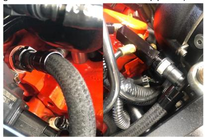
4. Connect the hose with no check valve to the PCV fitting in the lifter valley plate. Connect the shorter hose with the UPR check valve in it to the Procharger vacuum block using the UPR Plug and Play™ fitting.
