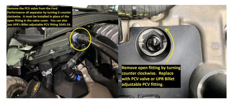
Remove the PCV fitting from the Ford Performance oil separator and swap it into the valve cover in place of the open fitting, or install UPR's Billet adjustable PCV fitting (5045-24) with the second to smallest jet.
