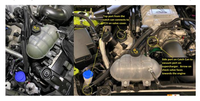
**4.** Install the UPR rubber braided hoses. The hose with no check valve in it connects from the PCV valve on the passenger valve cover to the top port of the catch can. Install the vacuum hose connecting the side port of the catch can to the vacuum port on the supercharger (with the arrow on the check valve facing away from the catch can towards the engine).
