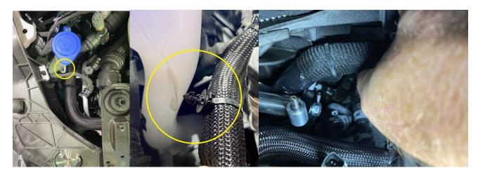
2. Remove the plastic retainer tree that attaches the coolant hose to the washer bottle. This will allow the hose to move and gain room for the catch can assembly. You may have to move the wiring harness over a little to allow the catch can to snugly drop in.
