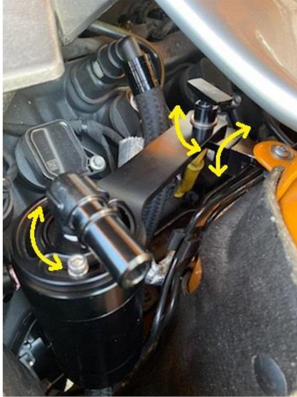
4. Connect the hose from the valve cover to the top fitting on the catch can. The Plug and Play fittings push in easily until it clicks. To remove, press the grey buttons on the fittings.
