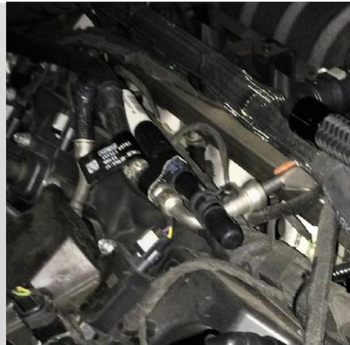
5. The hose with the check valve will be installed connecting the side fitting of the catch can to the vacuum fitting on the supercharger. The arrow on the check valve always faces away from the catch can.
