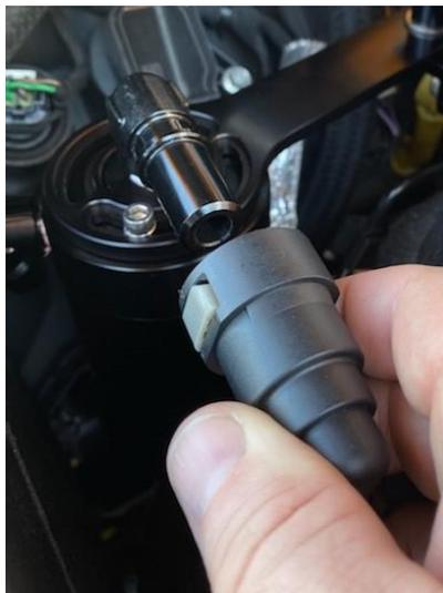
5. Connect the hose from side fitting on the catch can to the air inlet tube. NOTE: If running a turbo or centrifugal supercharger, this hose will connect to the air filter or air filter tube.
