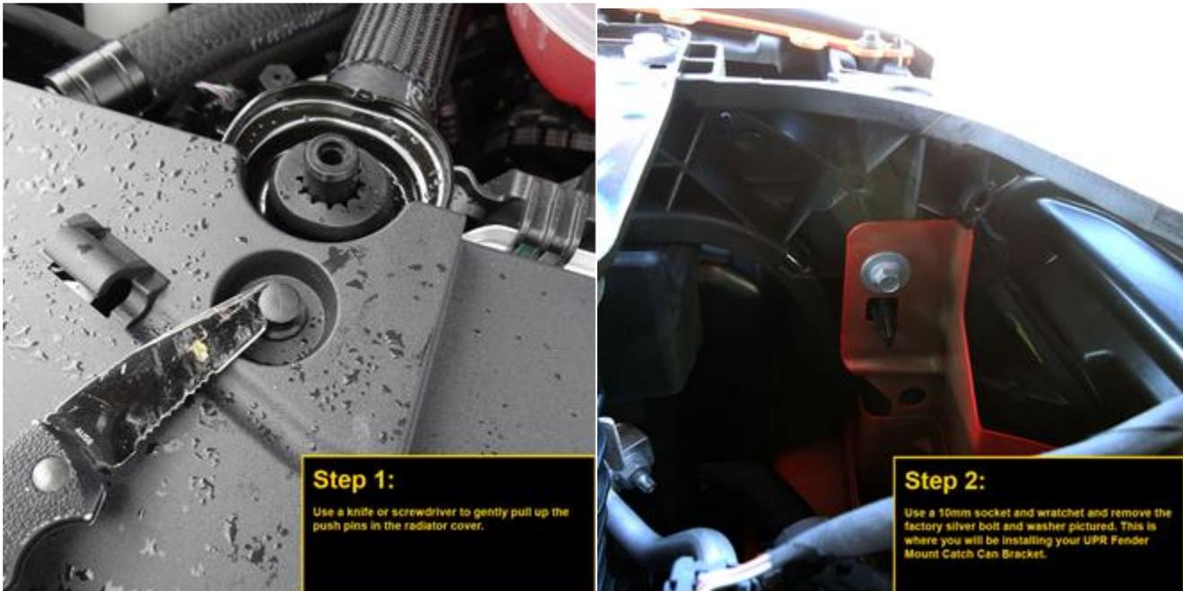
1. Use a knife or screwdriver to gently pull up push pins in the radiator cover, and remove cover.
