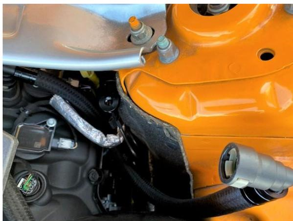
3. Install the Clean Side Catch Can onto the bracket with the supplied 10MM bolt ( or Knob if you selected the option). The allen head screws on top of the catch can, along with the bracket allows the can to be 'clocked' into many positions to fit your application.
