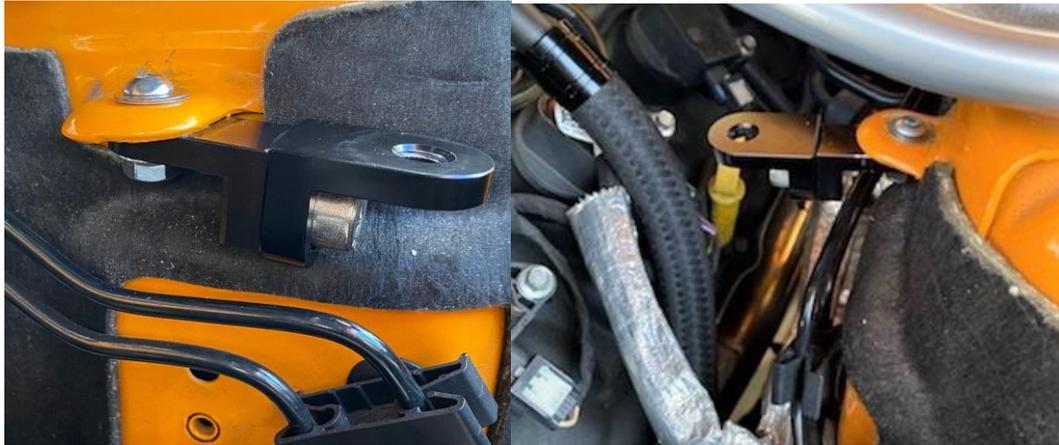
2. Install the 22" hose onto the driver side PCV fitting. Route the hose 'down' towards the shock tower, and back up as shown. This will reduce the chance of kinking the hose. You may adjust the routing as needed.
