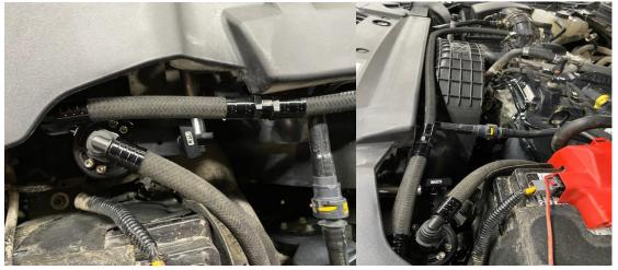
9. Remove the air intake tube by loosening the 2 band clamps, releasing the fitting, and the harness retailner.
