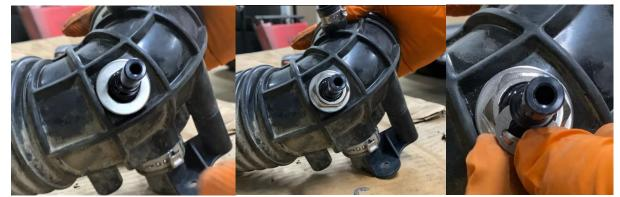
12. Reinstall the air intake tube, fitting, and harness retainer. Connect the WOT hose with the UPR Plug and Play fitting.
