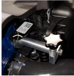
2. For best access to the PCV hose and connections, jack up and properly support the front of vehicle. Remove the driver side front wheel. Remove the 9 trim fasteners holding the access cover on, and remove the cover.
