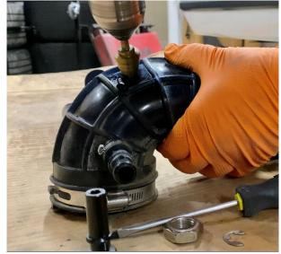
11. Disassemble the retainer clip, nut, and the washer from the Quick Tap fitting. Install the Quick tap fitting by pushing it up through the hole from the inside-out. Reinstall the washer, nut, then the retainer clip. Do not overtighten the nut. You can add a dab of RTV sealant to the base of the fitting before installing the washer if you made the hole a little too big.
