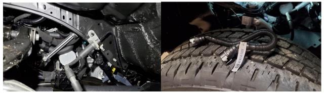
3. Position the coolant hoses down out of the way. You will look for the short, U-shaped PCV hose and feel for the connections. It will be nearly impossible to see the connections, so you will need to remove the PCV hose and install the UPR Catch can hoses on the engine by 'feel'.
