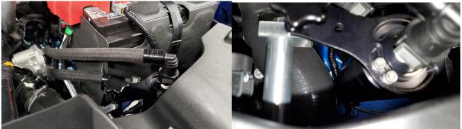
The Wide Open Throttle Hose will connect from the 90 Degree fitting on the catch can, and route along the fan shroud to the intake air box tube. Be sure the arrow on the check valve is facing away from the catch can. Route the WOT hose so that the fitting will comfortably reach the air intake tube. Mark the location to be drilled.
