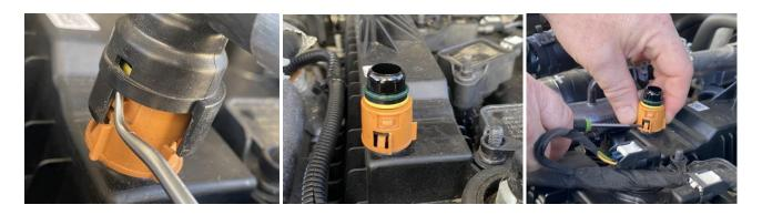
Now that you can see the 3 tangs, while applying upward pressure, use a pick or small screwdriver to release them and remove the rest of the fitting from the valve cover.
