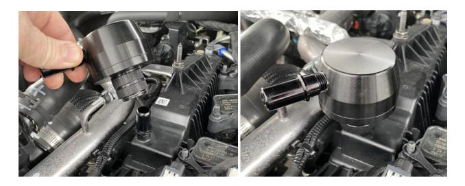
13. Install the 3 way fitting onto the Turbo Inlet tube. Be sure the male portion of the fitting is facing up. Connect the CCV tube to the male part of the 3 way fitting. Connect the WOT hose to the female portion of the fitting. Finally, connect the CCV tube to the Clean Side Separator.
