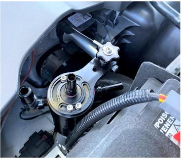
7. The 'Dirty side' hose from the PCV has a 90 degree fitting, and will connect to the top of the can. The 'Clean side' hose has a straight fitting with check valve in line will connect to the side of the can with the straight fitting.
