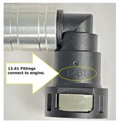
4. The UPR PCV hose, and Vacuum hose will have special fittings which will connect to the PCV and Vacuum fittings on the engine. The fittings can be identified by the '12.61' printed on the side of it.
