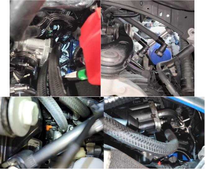
Route your hoses from where the catch can will be mounted, down past the throttle body so you can then route them to the fittings on the engine. The 'Clean side' hose (vacuum) will have a check valve installed in it, while the 'Dirty side' hose (PCV) will have no check valve. The arrows on the check valves always face away from the catch can.
