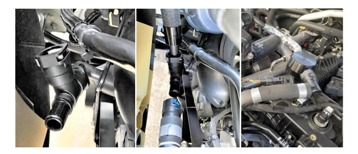
Go back over the installation to ensure there are no loose fittings, the catch can mount and bracket are secure and tightened, and all hoses are routed away from any sharp edges or hazards.
