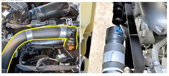
Disconnect the harness from the sensor on the Crankcase vent tube.
