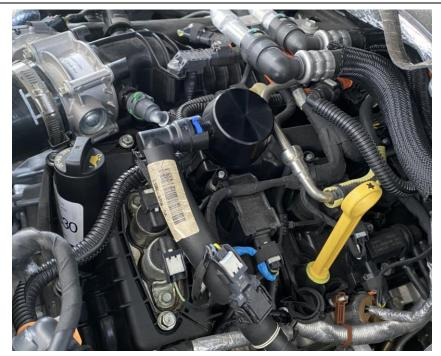
Install the Clean Side Separator onto the driver side valve cover CCV fitting by lifting up on the collar at the base of the CSS, then push the CSS onto the male fitting until it clicks firmly into place.
