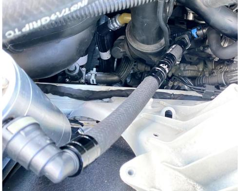
(The fitting at the catch can has been changed to a 45 degree fitting for better routing)
