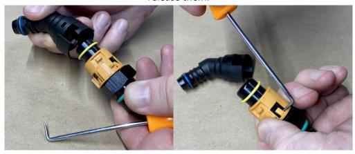
To replace the fittings on your factory CCV tube, use a heat gun or lighter to gently warm the plastic tube – do not melt or burn the tube. Pull the fitting out of the tube once it is warm, and insert the new fitting into the tube while it is still warm (caution: it will be hot). The tube will conform to the fitting as it cools. To assist, you can wrap a small zip tie around the tube end while it cools.
