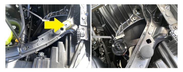
Find the un-used factory hole in the radiator support just to the right of the hood bumper. Mount the catch can with the provided hardware. You will need a 5/32 allen wrench.
