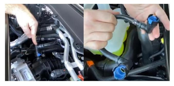
Locate the factory PCV hose that runs from the passenger valve cover to the intake manifold vacuum port.
