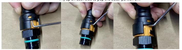
Now that you can see the 3 tangs, while applying upward pressure, use a pick or small screwdriver to release them.
