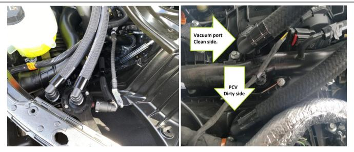
The longest hose with the check valve in it will be the 'Clean Side' or vacuum hose. When routing the hose, be sure the arrow printed on the check valve faces away from the catch can.
