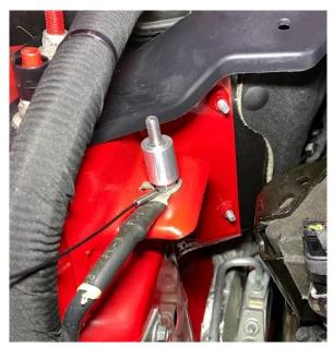
1. Locate the ground wire connected to the passenger side shock tower tab. Use an 8mm socket to remove the factory bolt. Thread in the supplied 6mm stud, then slide the catch can knob lanyard over the stud and lock it down with the supplied jam nut as shown. Finally, slide the supplied spacer over the stud. (*The ground wire must touch the body, do not install on top of the mount*)
