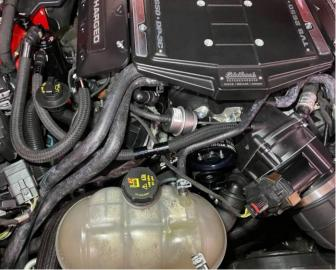
4. Install the Clean / Vacuum hose. Start by putting a small amount of engine oil on the male fitting on the supercharger inlet. Slide the supplied hose collar over the end of the hose and firmly push it onto the male fitting. Route the hose the connect to the side fitting on the catch can.
