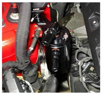
2. Install the passenger side catch can (shorter bracket than driver side) onto the stud with the supplied knob as shown.
