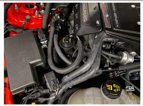
3. Install the Dirty Side hose. This hose will have a 45 degree fitting that will connect to the top of the catch can, and a 90 degree fitting that will connect to the PCV valve on the valve cover. Route the hose forward and loop back to the PCV as shown. You can rotate the fittings in the hose for the best fit.
