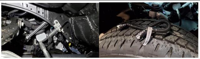
3. Position the coolant hoses down out of the way. You will look for the short, U-shaped PCV hose and feel for the connections. It will be nearly impossible to see the connections, so you will need to remove the PCV hose and install the UPR Catch can hoses on the engine by 'feel'.
