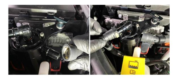
5. Install the UPR catch can onto the 90-degree billet bracket with the supplied bolt. Install the UPR Plug N Play<sup>™</sup> Fittings onto the catch can. The 'Dirty' side hose will connect to the Top of the catch can. The 'clean' side hose will connect to the right side of the catch can.
