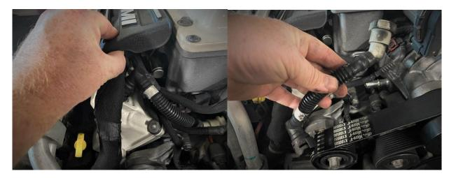
1. Lift the passenger side Plastic engine cover to gain access to the PCV tube. Remove the PCV tube by pressing the release buttons on the fittings. DO NOT PRY THE FITTINGS.
