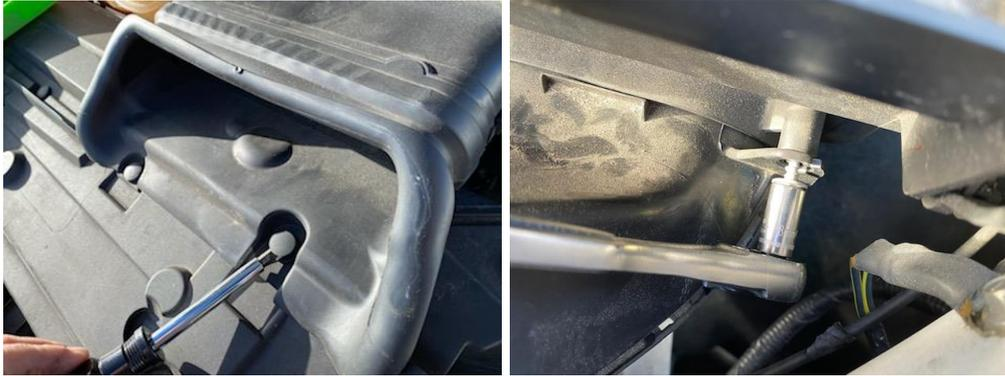
2. Locate the oval shaped hole in the frame on the driver side directly below the air inlet. Install the 90 degree mounting bracket to the frame with the supplied hardware. The bracket should be facing upwards. Install the catch can onto the bracket with the supplied hardware.
