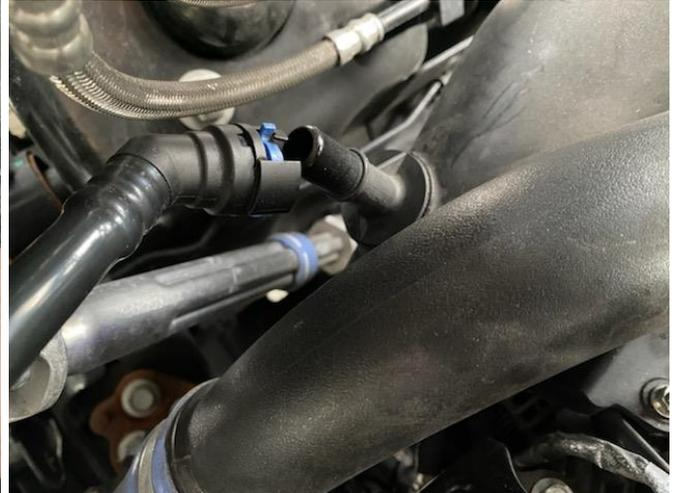
7. Connect male portion of the 3-way fitting into the CCV tube, and connect it to the turbo inlet tube as shown. The male end of the fitting should face the rear of the engine compartment.
