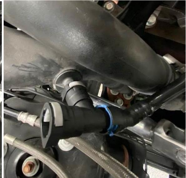
8. Install the CSS onto the Valve cover fitting by lifting up on the collar at the base, and then pushing down on the CSS. The collar will click when fully engaged. Turn the factory fitting in the CCV tube to enable it to connect to the CSS.
