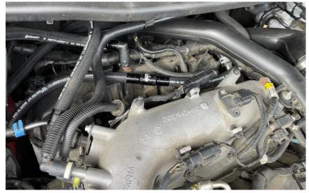
3. The longest hose in the kit will be the Wide Open Throttle (WOT) hose. Route the hose between the intake manifold and the rear valve cover as shown. The check valve in the hose will have an arrow printed on it. The arrow must face away from the catch can, towards the intake tube connection. Connect the UPR Plug N Play fitting to the UPR air intake tube. Route the other end of the hose to the far side of the catch can.
