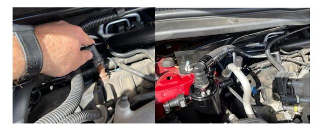
4. Locate the factory PCV tube that runs from the rear valve cover to the intake manifold vacuum port and remove it. The hose with no check valve will connect from the PCV on the valve cover to the **top** fitting on the catch can.
