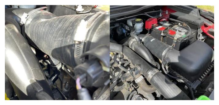
Remove the factory rubber intake tube and replace with the UPR tube. The fitting should face down. Leave the air box lid loose so it is easier to access the fitting. If you have an aftermarket cold air intake, you may need to cut the UPR tube to length.
