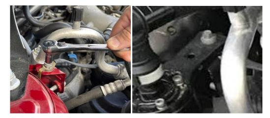
1. Disconnect the negative battery cable. Use an 8mm socket to remove the ground strap bolt on the passenger shock tower. Install your UPR catch in this location and secure with the ground bolt.
