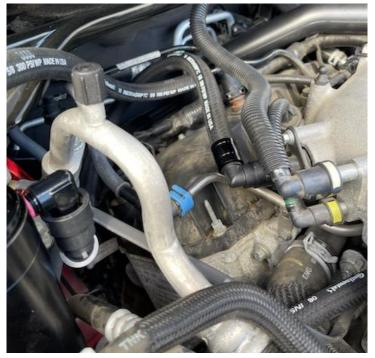
5. The last hose is the vacuum hose. The **arrow** on the check valve in this hose **must face away from the catch can**, towards the intake connection. Route the hose from the intake manifold towards the rear of engine compartment, then back to the catch can. Route it so that there are no kinks in the hose.
