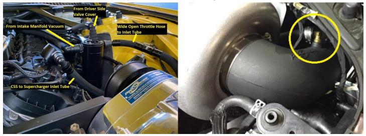
Check your UPR Catch Can every 500 miles at first to get a feel for your vehicle's needs. Always check and drain the catch can more often in winter / freezing weather. If the water/oil mixture in the catch can is allowed to freeze it will cause damage to the catch can and internal components. Any damage due to freezing is NOT WARRANTY.
