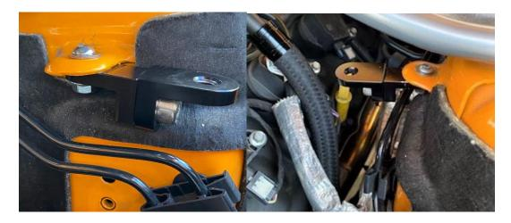
2. Install the Catch Can onto the bracket with the supplied 10MM bolt (or Knob if you selected the option). The allen head screws on top of the catch can, along with the bracket allows the can to be 'clocked' into many positions to fit your application.
