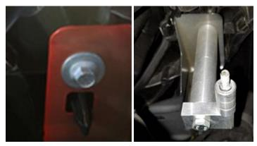
2. On the driver side of the front of the car, remove the 10mm bolt that is just to the right of the radiator on the radiator support. Install the UPR bracket in its place.
