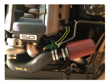
6. The Clean Side Separator will connect to the driver side valve cover. Pull up on the collar at the base of the CSS before pushing it onto the valve cover fitting. It will click when secured. Route the hose to the fitting on the supercharger inlet tube (cold air kit). If your kit has a T fitting connecting to this inlet tube, cut the hose to fit and connect the CSS to the T. \*On Gen3 Paxton / Vortech kits, it may be necessary to modify or space the coolant tank brackets to clear the CSS.
