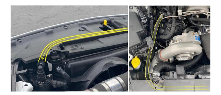
4. The hose with NO check valve in it will route from the top fitting on the catch can, across the front of the radiator (under the cover) to the Passenger side valve cover PCV fitting.
