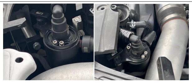
3. Mount the UPR catch can to the bracket with the supplied knob. You can loosen the allen screws at the top of the catch can to enable clocking of the catch can for the best fit.
