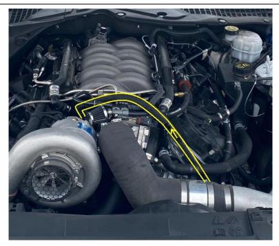
5. Route the hose with the check valve in it from the side of the catch can to the intake manifold vacuum fitting. The arrow on the check valve must face away from the catch can towards the engine.
