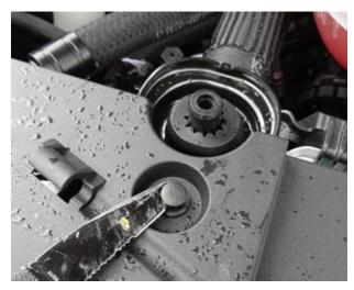
1. Use a knife or screwdriver to gently pull up push pins in the radiator cover and remove the cover.
