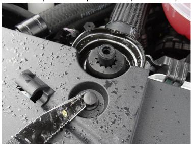
2. Use a 10mm socket and ratchet to remove the factory silver bolt and washer pictured. This is where you will be installing your UPR fender mount catch can bracket. Install the bracket and tighten it so that it is oriented with the stud facing up as shown.
