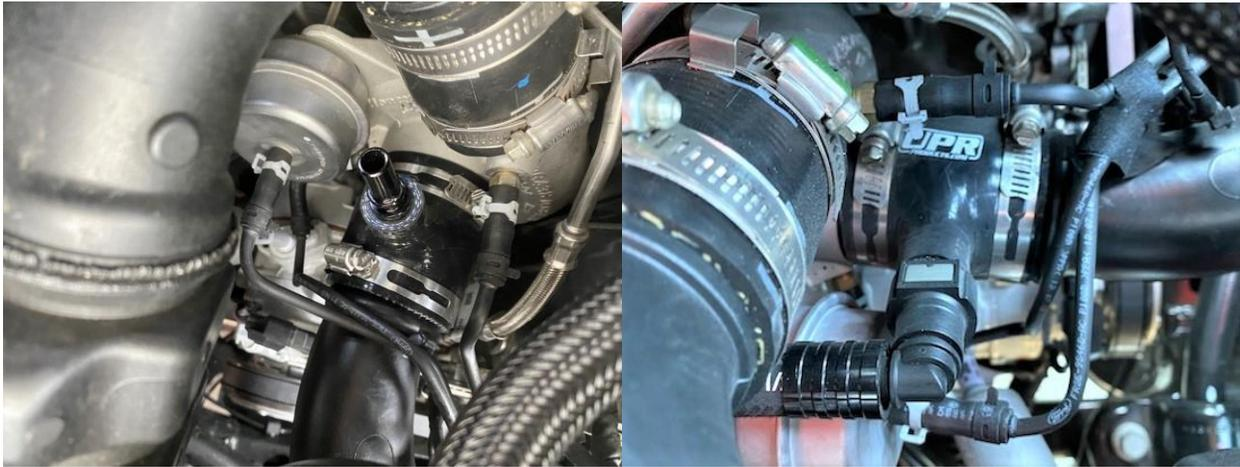
Install the UPR Turbo inlet coupler. Leave it loose until you clock it for the best fit with the WOT hose and the UPR Plug N Play™ male fitting. Route the UPR WOT hose so that the arrow on the check valve faces away from the catch can towards the coupler.
