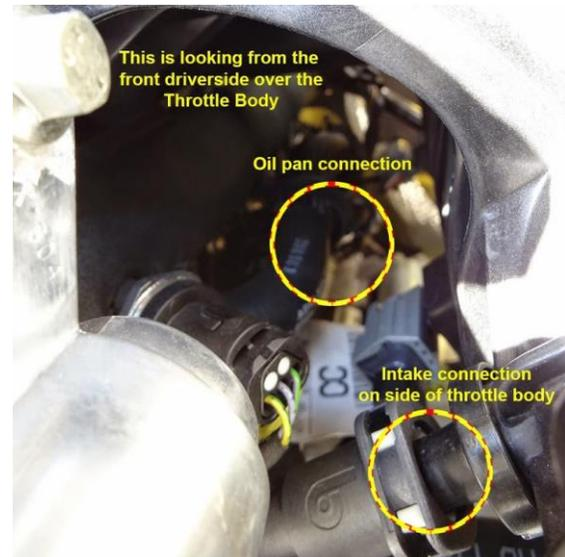
Locate the Factory PCV tube. It connects the Vacuum Port just behind the throttle body to the PCV port on the driver side of the engine block just above the oil pan. Remove the tube by pushing the button on the side of the fittings.
