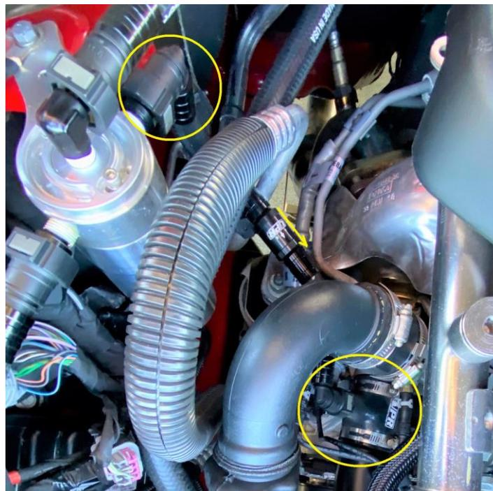
Go back over all of the connections and hoses to make sure they are secure. Be sure the coupler is tightened.
