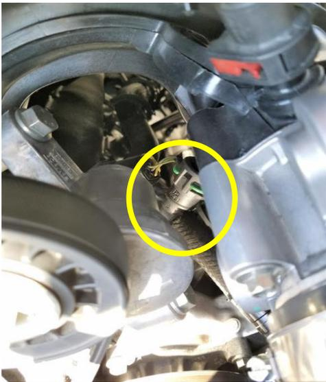
Locate the vacuum or 'Clean Side' hose in the kit. It is the longer of the 2 hoses with a check valve installed. Connect the UPR Plug N Play™ 90 degree '12.61' fitting on this hose to the vacuum port just behind the throttle body. The hose will be routed towards the front of the car.
