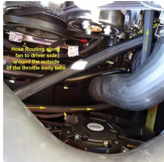
Route the hose so the arrow on the check valve will face away from the catch can, towards the engine. Be sure to route the hose so it does not contact any pulleys or other hazards. Connect the catch can end of the hose to the forward facing port on the catch can.
