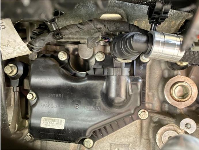
The hose in the kit without a check valve is the hose for the 'Dirty Side' PCV connection. The 90 Degree '12.61' fitting goes to the PCV on the side of the block. Connect this hose to the factory PCV fitting by making sure it is pushed all the way onto the PCV. It will click when properly engaged as shown.
