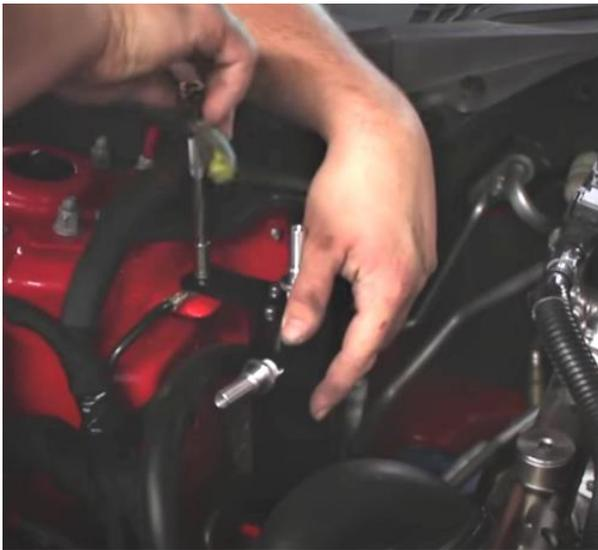
Mount the UPR Dual Valve catch can to the passenger side strut tower using the ground strap bolt as shown. Removing the air box tube will make reaching the vacuum tube and hose routing easier to access
