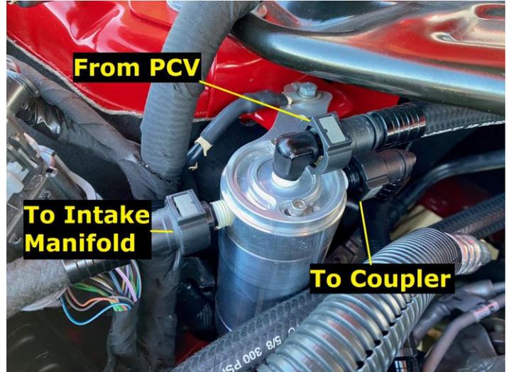
Route the dirty side PCV hose behind the engine, over the transmission bellhousing area to the top inlet fitting of the catch can.
