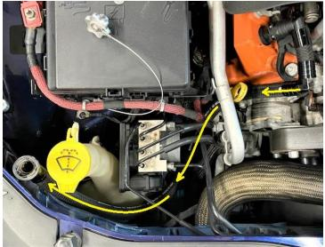
**5.** Using the longest hose in the kit, route the open end of the hose from the passenger side of the engine compartment, behind the supercharger, and out on the driver side of the engine.
