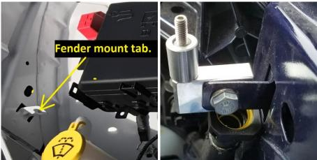
2. Unclip the battery cable between ABS and fuse box covers to remove ABS cover for routing hoses.
