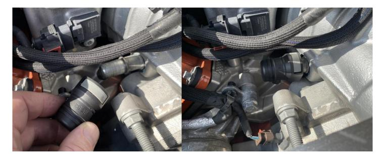
**10.** You can use the remaining rubber cap to cap off the driver side crankcase vent sensor fitting if equipped. With this Race style breather tank, the sensor will need to be eliminated from the tune to avoid a check engine light.
