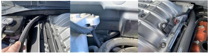
**6.** Route the end of the long hose with the 45 degree fitting installed between the fuse box and ABS controller. Properly routed, the hose will fit under the factory engine cover.
