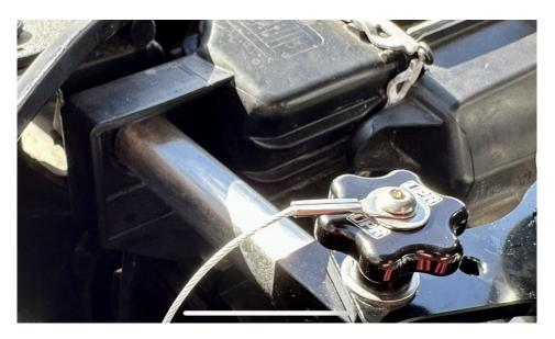
1. Remove the bolt at the top driver side of the radiator mount. Install the UPR bracket with the supplied bolt.
