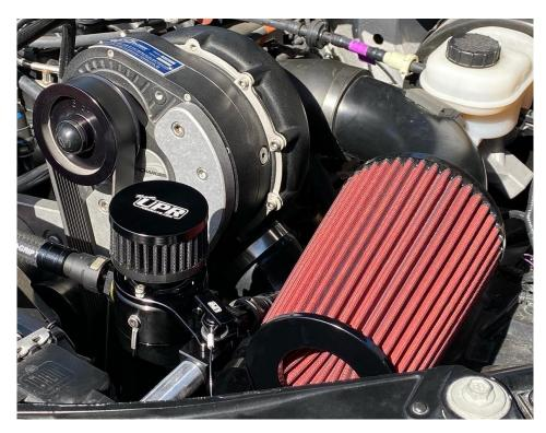
2. Install the UPR breather tank onto the bracket with the supplied Knob. The allen screws on the top bracket can be loosened to allow you to clock the breather tank into the best position. Tighten the screws and knob once you are happy with the fit.
