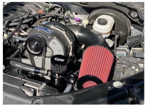
Always check and drain the catch can more often in winter / freezing weather. If the water/oil mixture in the catch can is allowed to freeze it will cause damage to the catch can and internal components. Any damage due to freezing is NOT WARRANTY. You must dispose of the liquid collected in the catch can properly (with used waste oil) properly according to your local laws.
