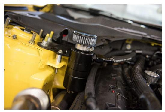
2. You are going to attach the 5/8 braided hose with the built in T to the can. The shorter line will connect to that side of the valve cover that is closest to the can.
