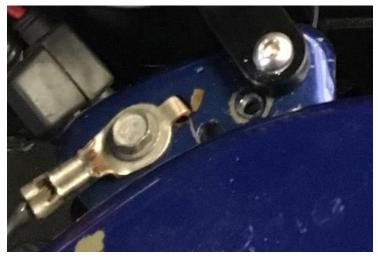
Mount the bracket with supplied bolt to the former ground hole. You can make another hole if you would like
