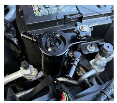
2. Attach the catch can to the UPR billet bracket with the supplied knob. You can leave the catch can slightly loose to allow adjustment when routing hoses. The allen screws at the top of the catch can allow for adjustment as well. Once the hoses are routed, adjust the catch can for best fit and tighten fasteners.
