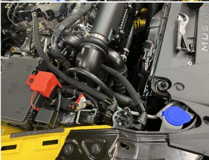
**10.** Install the last hose. Starting at the clean side catch can, connect the 45 degree fitting to the front facing fitting on the catch can. Connect the other end ( 90 degree fitting) to the air inlet tube where the factory hose had been connected.
