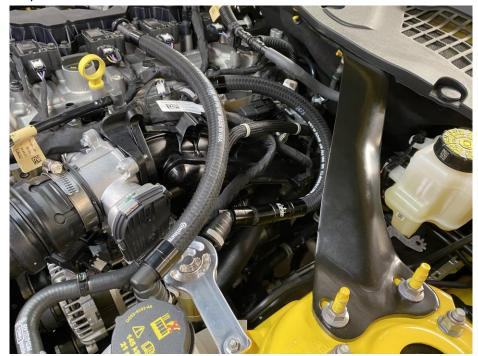
**4.** Install the UPR PCV hose. The straight fitting will connect to the PCV manifold, and the 90 degree fitting will connect to the front facing fitting on the catch can as shown.
