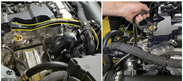
**8.** Locate the crankcase vent hose and remove it. It will connect from the passenger side of the PCV manifold on the valve cover to the air intake tube. Move the fitting retainer to the side and slide the fitting off.
