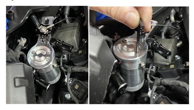
**6.** Locate the factory PCV hose that connects the PCV valve on the passenger side valve cover to the intake manifold vacuum fitting. If your engine is equipped with a cover, lift the cover to access the fitting behind the throttle bodies. Remove the hose by sliding the tabs on the fittings to the side and lift it off.
