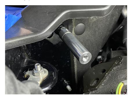
**4.** Install the bracket extension and 90 degree bracket using the supplied 6mm x 50mm long bolt. Be sure the short side of the 90 degree bracket is facing up. Tighten the bolt with a 10mm socket to secure the bracket.
