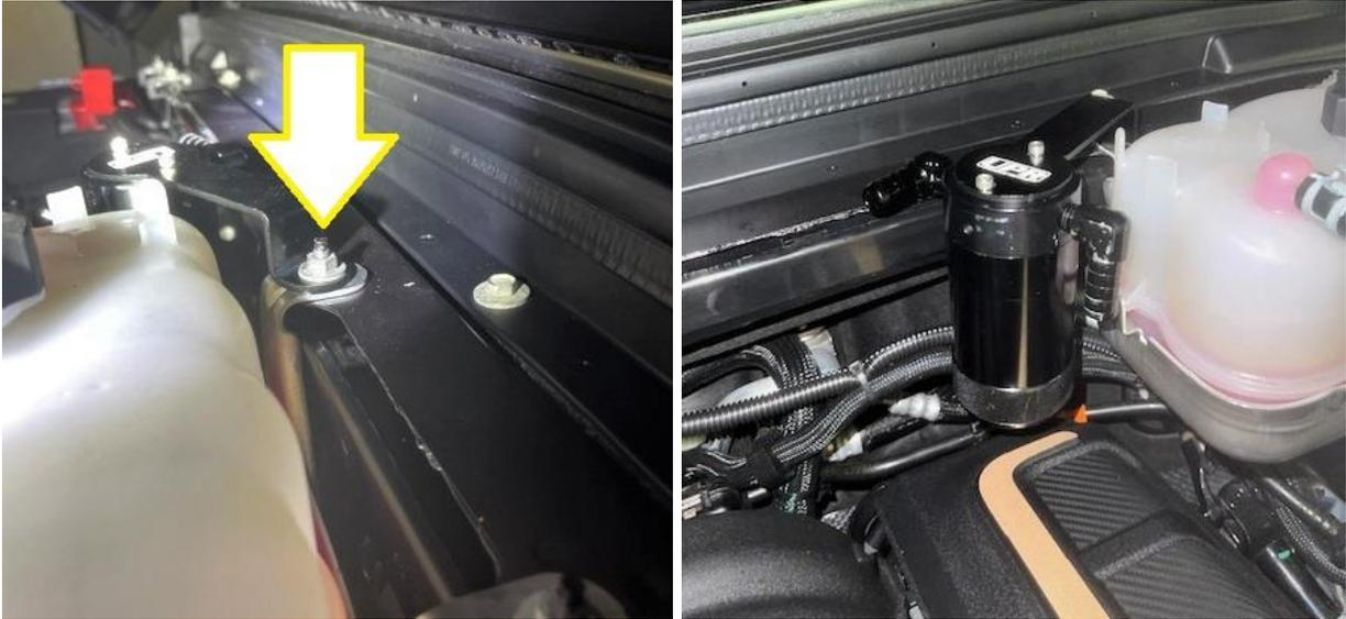
1. Remove the nut from the coolant degas bottle bracket, install the UPR catch can bracket and reinstall the nut as shown.
