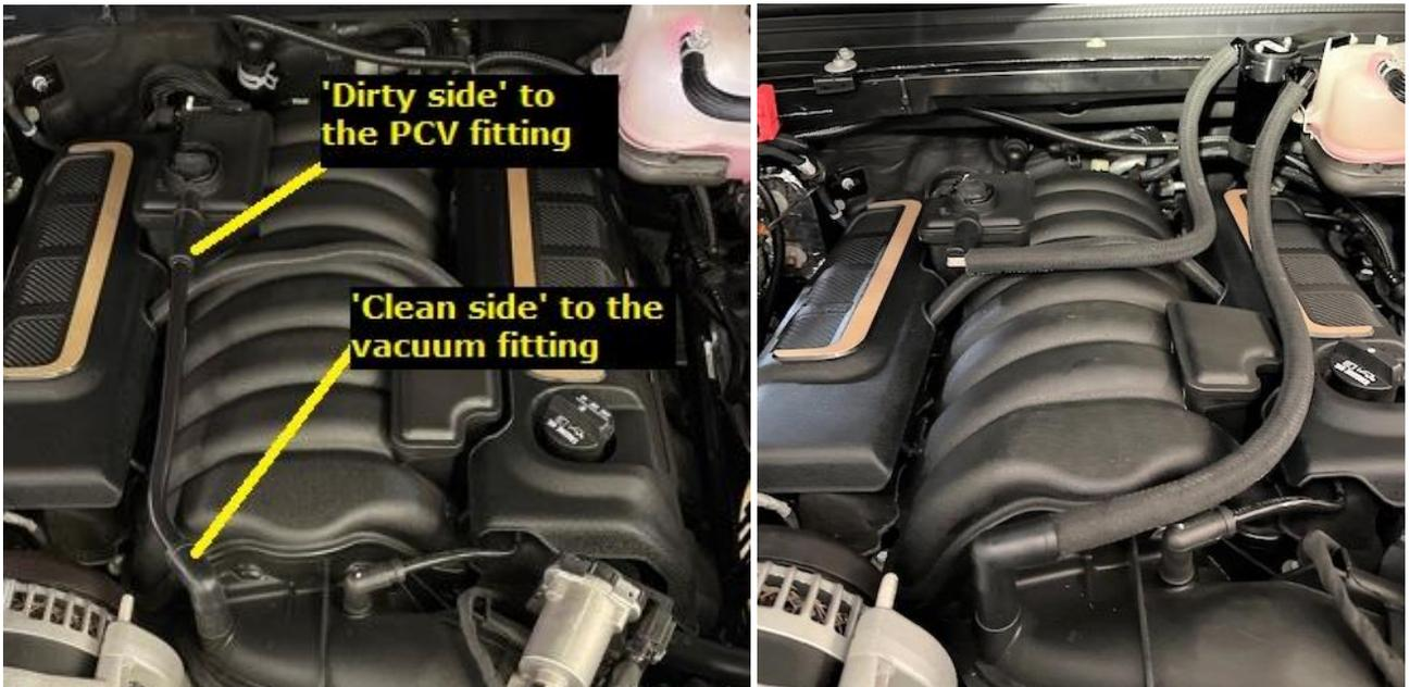
2. Locate the factory PCV hose and remove it from the rubber boots. Connect the hoses to the catch can as shown with the supplied adapter fittings.
