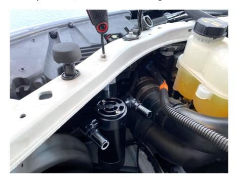
1) Find the un-used factory hole in the radiator support just to the left of the hood bumper. Mount the catch can with the provided hardware. You will need a 5/32 allen wrench.
