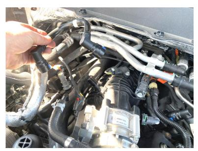
2) Locate the factory PCV hose. It runs from PCV on the passenger valve cover to the intake manifold vacuum port. Remove the hose. Keep the hose in case the vehicle is to be put back to stock.
