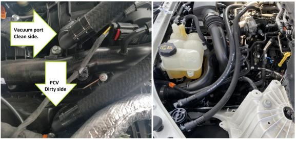
4) Connect the Dirty Side hose from the PCV on the passenger side valve cover to the inlet fitting on the catch can. Route the hoses so they are clear from hazards like belts, fans or exhaust.
