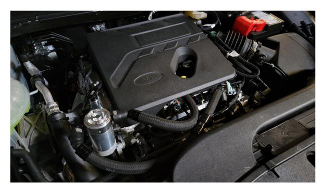
10. Check the catch can about every 500 miles until you get a feel for how much liquid your engine will produce. It'll be easy to service by unhooking the Plug N Play connections and wingnut, then unscrewing the bottom of the can. The containment cup does not need to be excessively tightened, just snugged.
