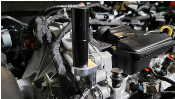
5. Place the catch can assembly onto the bracket and tighten the wingnut.
