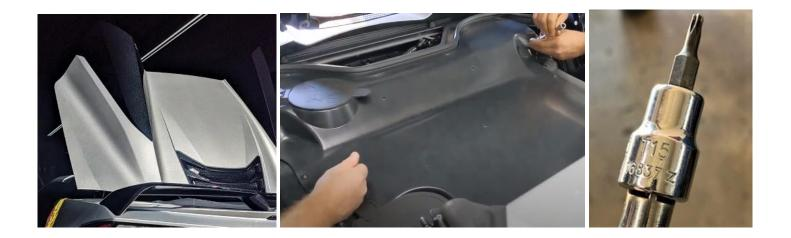
1. Raise the convertible top lid to gain access to the engine cover. Use a T15 torx bit to remove the engine cover fasteners. Lift the engine cover off (it's light but is best done with 2 people) and set it aside.
