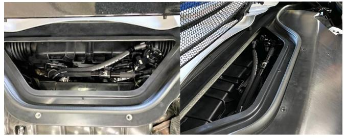
When servicing the catch can, you will reach in through the rear vent opening with the convertible top lid up. Release the UPR Plug N Play fittings by pressing the buttons on the sides and slide them off. Never pry the fittings. Check the catch can every 500-100 miles until you have a good feel for how often yours will need to be serviced, all cars are different.
