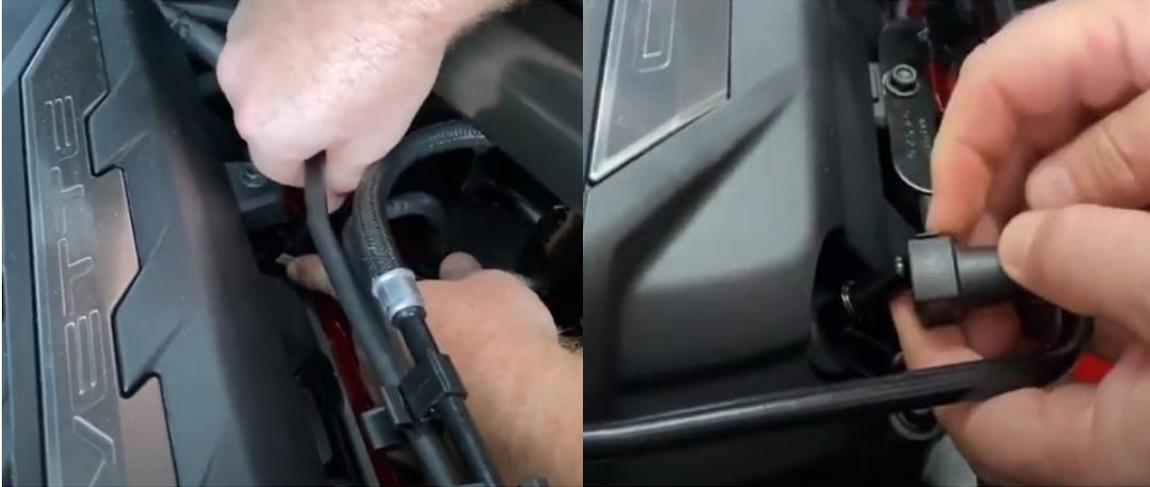
1. Remove the factory PCV hose. The hose runs from the vacuum port on the intake manifold to the PCV fitting at the lower front passenger side of the intake. It is easily released by pushing the buttons on the side of the fitting.
