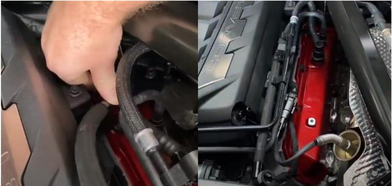
2. The UPR PCV hose will be the shorter of the two in the kit. Install the hose onto the PCV fitting and route it to the rear of the engine as shown. The hose can be secured with the factory looms. The hose end fittings are not crimped, so they can be rotated as needed.
