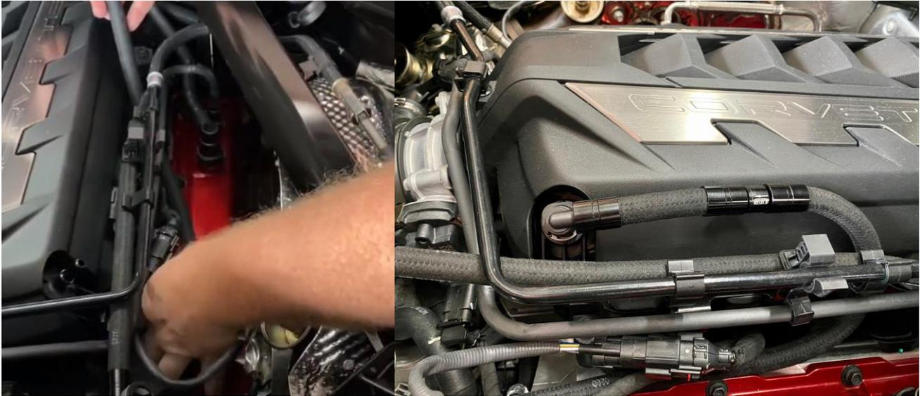
3. Route the UPR Vacuum hose behind the PCV and Fuel lines, close to the intake, and loop it towards the rear of the car. The check valve in the hose has an arrow printed on it. The hose must be routed so that the arrow points towards the engine, away from the catch can.
