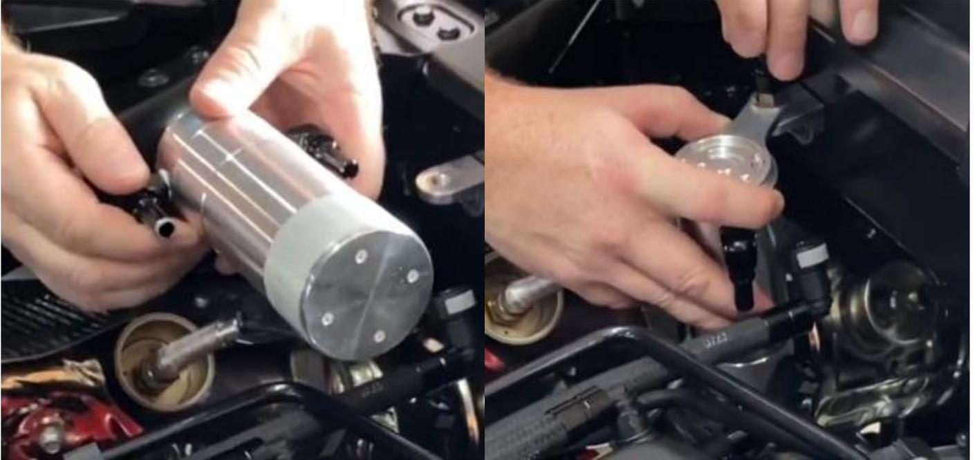
5. The catch can outlet will be indicated by a silver marking on the barrel of the fitting. This side of the catch can will connect to the intake manifold vacuum hose. ( the one with the check valve in it.) Install the UPR catch can onto the billet bracket with the supplied 10mm Allen bolt, or optional quick release knob if it was selected.
