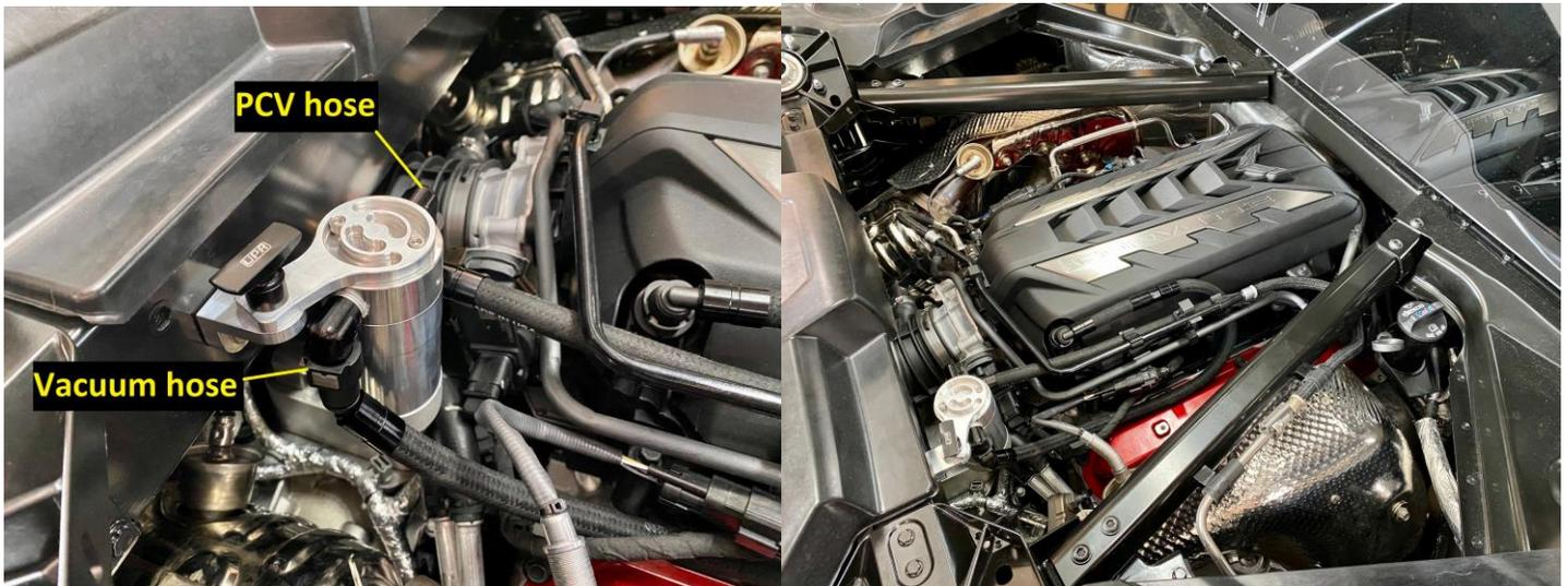
6. Connect the vacuum and PCV hoses to the catch can. The UPR Plug N Play connectors will simply clip on just like the factory connectors. To release them, Push both grey buttons on the fitting and slide it off. The catch can will be easily serviced by disconnecting the Plug N Play fittings, unscrew the catch can from the mount, and dispose of the liquid by unscrewing the containment cup to dump it out. Always dispose of the liquid like you would used oil.
