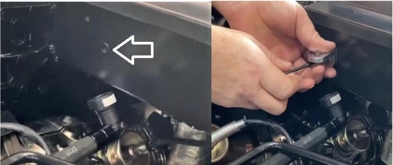
4. On the rear crossmember, there are 2 threaded holes. Using the supplied hardware, install the UPR Billet 90 degree bracket onto the rear crossmember using the lower, inboard hole as shown
