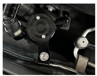
2. Install the catch can onto the bracket with the supplied hardware. You can loosen the allen screws on the top of the catch can to allow you to turn and clock the can for the best position.
