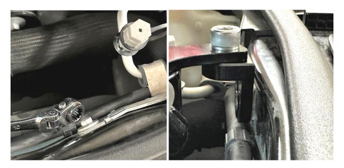
1. Locate the 10mm bolt holding the AC line bracket on the driver side of the front radiator support and remove it. Install the 90 degree bracket in this location with the supplied bolt (bolt may vary from picture). Be sure the short side of the 90 degree bracket is facing up.
