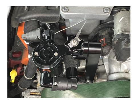
4. Mount the catch can to the bracket. Connect the PCV side hose to the front facing fitting on the catch can by running the hose under the bracket as shown. Connect the remaining hose that is connected to the supercharger vacuum fitting to the other side of the catch can.
