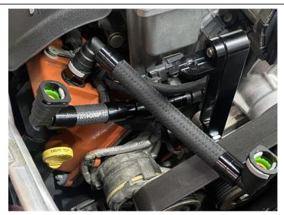
3. There are 2 hoses in the catch can kit. The hose with 90 degree fittings on both ends is the PCV side hose. The hose with a 90 and a straight fitting is the supercharger side (straight fitting connects to the supercharger vacuum fitting). Connect the hoses as shown before mounting the catch can.
