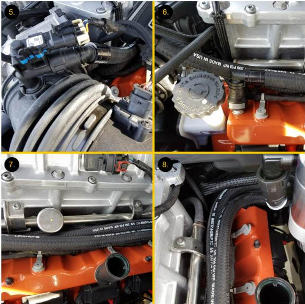
5. Mounting clean side hose with the 45 deg fitting to the intake tube.
