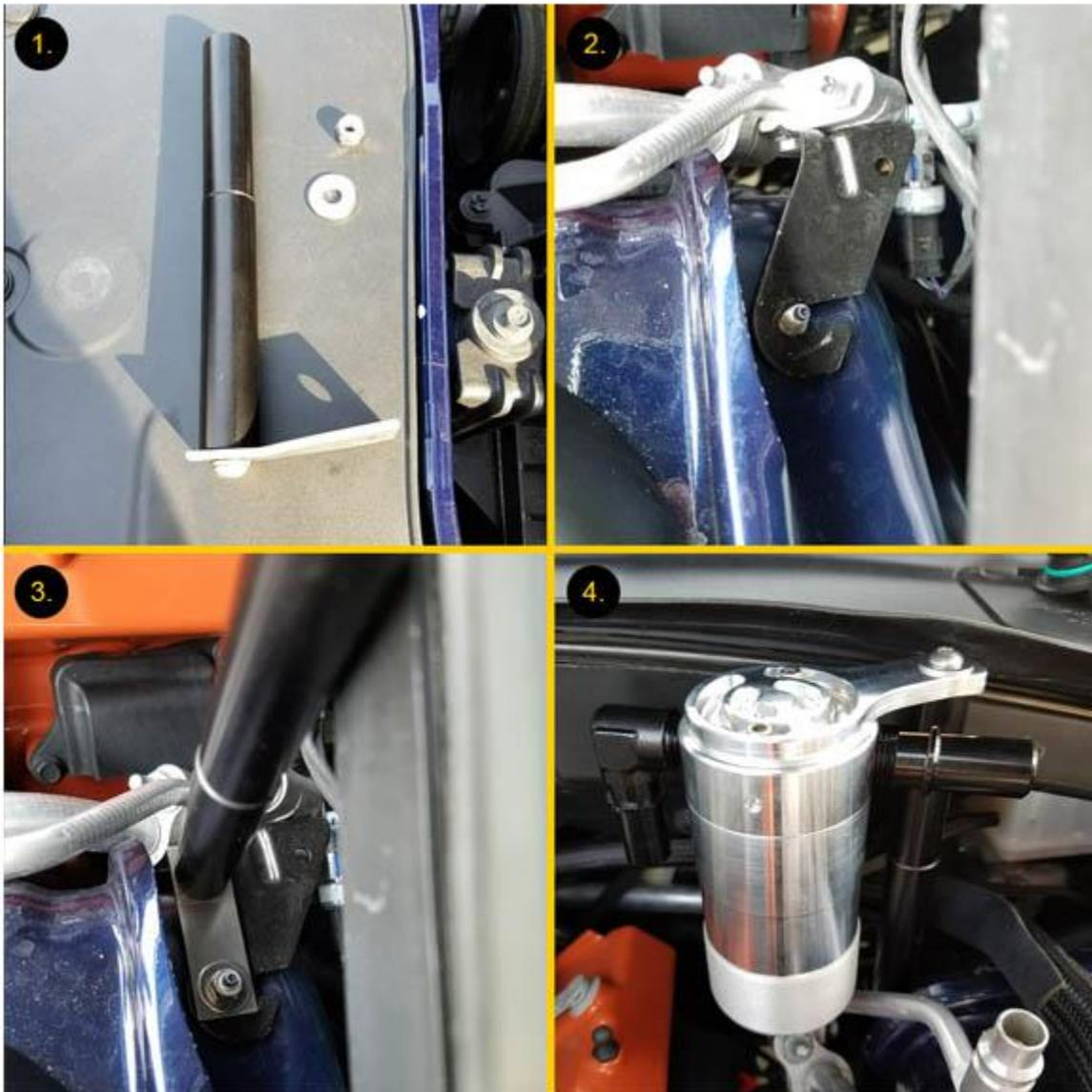
1. Mounting bracket with nut and lock washer
