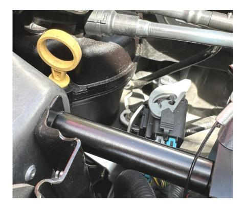
Remove the bolt from the passenger side hood hinge bracket and install the supplied bracket. (*The bracket shown is a prototype so your bracket may look different*)
