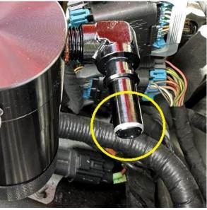
Click the UPR Plug and Play hoses onto the catch can. The outlet to the intake manifold vacuum fitting will be closer to the firewall and will be marked with a silver ring around the end of the fitting. If you selected to add a check valve to your kit, it will be installed in the vacuum hose. Be sure the arrow on the check valve is facing away from the catch can, towards the engine.
