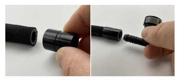
If your Corvette has quick connect fittings on the factory hose, remove the hose by releasing the tab on the fittings and remove the hose. Install the UPR billet hose end ferrules, then push the quick connect fittings into the hose. (sample hose end installation is shown, your fittings will be a different angle)
