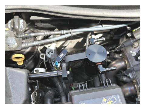
Install the UPR catch can onto the bracket.
