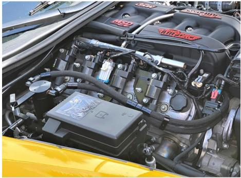
Route and secure your catch can hoses as needed to avoid contact with hot exhaust or other hazards.
