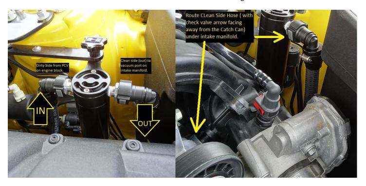
Always check and drain the catch can more often in winter / freezing weather. If the water/oil mixture in the catch can is allowed to freeze it will cause damage to the catch can and internal components. Any damage due to freezing is NOT WARRANTY. You must dispose of the liquid collected in the catch can properly (with used waste oil) properly according to your local laws.
