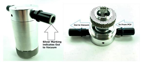
Note the silver ring on the outlet fitting. This indicates the outlet of the catch can which will connect to the intake manifold vacuum port. Another way to tell is to open the catch can and look for the outlet which is the machined 'C' shaped opening as shown.
