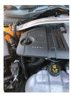
2. Remove factory oil cap from passenger side cover
