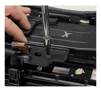
Use a 1/4" or larger drill bit to carefully drill out the melted over section of each locating pin. You only need to knock off the area that is melted. Do not drill into the grille assembly. Scrape off any remaining residue.
