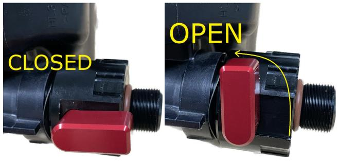
4. To use the drain valve, remove the billet dust cap by rotating counter clockwise. You can slide a 5/8 hose (not included) over the threaded end of the drain valve to control oil flow if you like. Turn the drain valve lever 90 degrees to allow oil to flow out.
