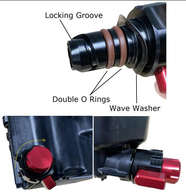
**3.** To install the oil drain valve, Be sure the wave washer is in place and insert the drain valve so that the drain lever is facing down towards the ground and rotate the valve body clockwise until it clicks. If you have the grooves in the valve lined up with the tangs in the oil pan, it will turn easily. If it is difficult to turn, stop, and recheck the alignment to prevent damage to the oil pan.
