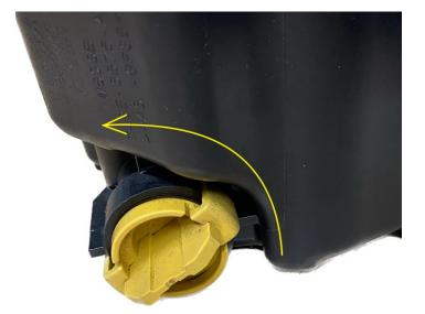
Be sure the engine is cool, and you have a proper oil drain pan in place before removing the drain plug. Remove the factory drain plug by rotating the yellow plug counter clockwise.
