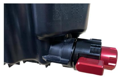
**5.** When the oil is drained, turn the valve back to the closed position and reinstall the dust cap.
