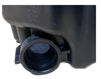
2. Once the oil has drained completely, wipe out the drain hole to remove residual oil.
