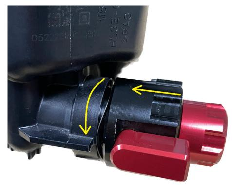
6. (Optional) To remove the drain valve, **push the drain valve in towards the oil pan** firmly **before turning counter clockwise**. Failure to push the drain valve body in towards the oil pan and / or using a wrench or other tools to turn the drain valve will result in oil pan damage.
