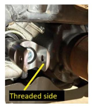
**Tech Tip:** If you do not have a 14mm Allen socket, you can make one from a 14mm headed bolt. Thread a couple of nuts onto the bolt and tighten them, or tack weld the nut, then you can use a 14mm deep socket with the bolt inserted to tighten the clevis bolt.
