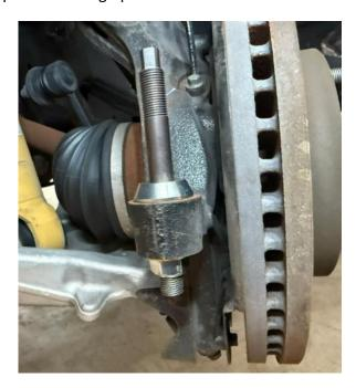
8. Install the new UPR steering rack boot onto the UPR aluminum tie rod sleeve:
