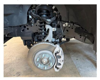
2. Lift the front of the truck and support it properly with appropriate heavy duty jack stands under the driver and passenger side frame rails. Remove both front wheels.
