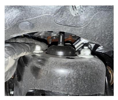
6. There are three 18mm nuts holding the upper strut assembly into the frame pocket. Loosen the nuts, but do not remove them entirely.
