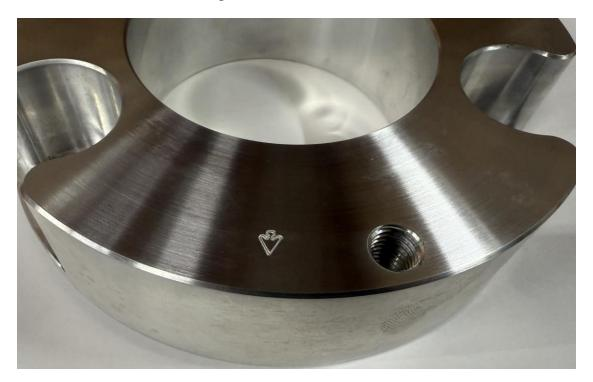
13. The UPR leveling spacer will be marked with an arrow. The arrow will face out towards the tire.
