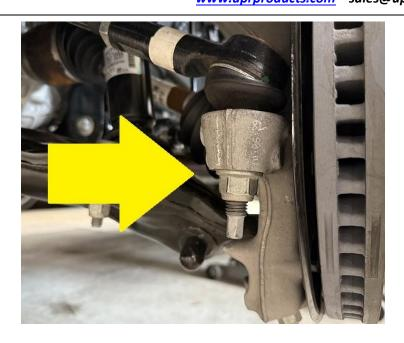
5. Remove the tie rod end link from the knuckle. Our 25 F150 had a 21mm nut on the tie rod end.
