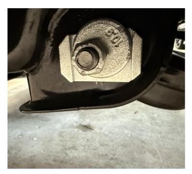
20. Install the cam nut onto the pivot bolt. Using a 27mm wrench or socket to hold the cam nut in place, tighten the pivot bolt until the cam nut is seated. You can set the pivot bolt position close to your marks as a base setting until you get to an alignment shop. Tighten, but do not torque the bolts at this time.
