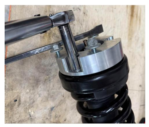
15. Install the leveling spacer onto the strut so that the arrow stamped on the spacer will face out towards the tire. Use the provided nuts to install the leveling spacer onto the strut. Torque the nuts to 30 lb-ft.
