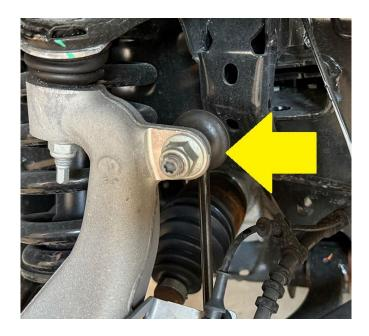
4. Remove the sway bar end link from the knuckle. Our 25 F150 had a 21mm nut and the stud had a T45 Torx.
