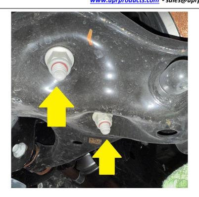
7. There are 2 nuts holding the lower strut assembly to the lower control arm. Remove the nuts with an 18mm socket and set them aside.
