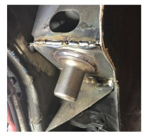
4. Weld the mount in to the body. We recommend that once you are finished to tape off the threaded stud and paint the area to prevent rust.
