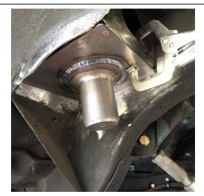
3. Line up the spring mount on the car, some trimming may be necessary. Adjust the position of the plate to best align the upper mount with the spring perch of the control arm you are using. Prep the area you will be welding in. Cover the threads to prevent damage from weld splatter.
