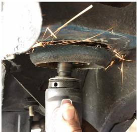
2. Cut out the factory upper spring mount with a cut off wheel. Use a grinder to smooth the area flat.
