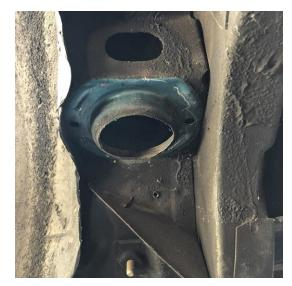
1. Remove your factory rear springs so you have room to work on the upper spring perch area.
