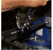
Using two sets of pliers work the shield apart until you can remove it from the shaft of the shock. Another option would be to cut the shield on the side as we did we step 3.
