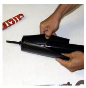
To use the Strange shocks with this coil over kit the dust shields have to be removed. Using a razor knife make a cut from the bottom of the shield to the top. (Fish style razor not included!)
