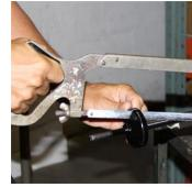
Next make a cut in the metal dust shield with a hack saw or cut off wheel.
