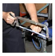
The dust shield is held on with two small tack welds and both must be cut.
