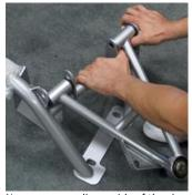
Now you can pull rear side of the A-Arm in place to align with mounting holt holes.
