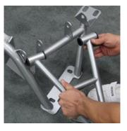
\* Start by installing the front side of the A-arm in front K-member slot at an angle. Stay well below the mounting bolt holes.
