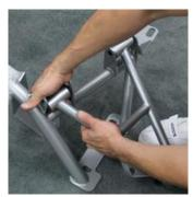
Lastly pull the front of the A-arm into place and align with mounting bolt holes.
