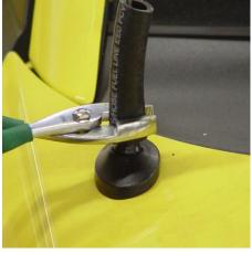
Install the new Billet Antenna and place a piece of rubber hose over the antenna as pictured. Tighten with a pair of pliers. The rubber hose will protect the antenna while tightening.
