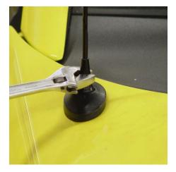
Using a wrench or adjustable wrench, remove the factory antenna.
