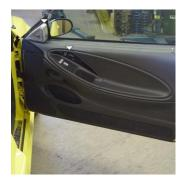
Remove the Mach 460 Speaker Cover & Window Switch trim. The speaker cover is removed by simply inserting a flat screwdriver between the cover and the speaker housing. To remove the window switch trim, insert a flat screwdriver between the trim and the door panel. The trim will simply pop out.
