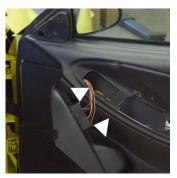
Remove the window switch retaining screws located on the back of the window switch assembly.
