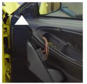
Remove the Mach 460 speaker by removing the retaining screw located inside the mark hole. See above picture.
