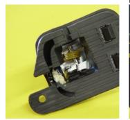
Position the billet door handle and the spring in place as pictured. Insert the new supplied door pin and the retaining screw. Make sure to use Loc-Tite or a similar product to prevent the screw from loosening.
