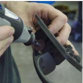
Using a dremel tool cut off the end of the retaining pins. This will allow the pin to be removed. Make sure to keep the door handle spring which will fall out once the pin is removed.
