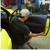
Carefully remove the inner door panel by lifting up and off.
