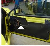
Using a drill, drill out the aluminum pop rivet that holds the factory door handle in place. NOTE: MAKE SURE THE WINDOW IS UP BEFORE DRILLING!!!
