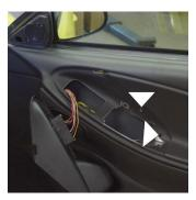
Remove the two door panel retaining screws using a Phillips screwdriver.
