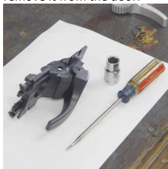
Slide the handle forward to remove it from the door.
