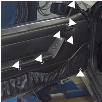
Remove the Phillips screws retaining the inner door panel.
