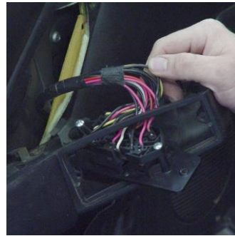
Route the window controls off of the inner door handle.
