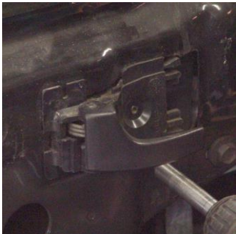
Remove the Phillips door handle retaining screw.
