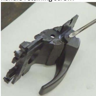
Remove the Phillips door handle retaining screw.
