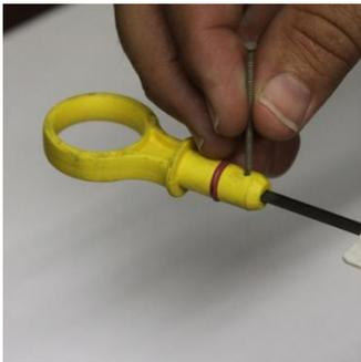
Using the paneling nail and hammer push the factory dipstick pin out of the handle releasing the handle from the dipstick.
