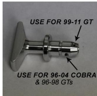
The Billet handle will have two holes in it for the pin. Use the correct hole based on your engine. 96-04 Cobras & 96-98 GTs use the top hole and 99-11 GTs use the lower hole.
