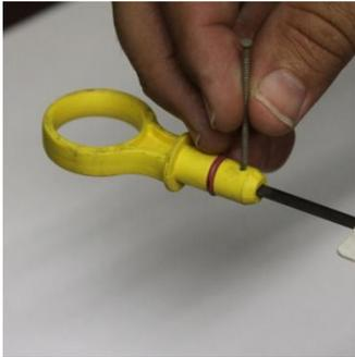
Using the included paneling nail and a hammer push the factory dipstick pin out of the handle releasing the handle from the dipstick.
