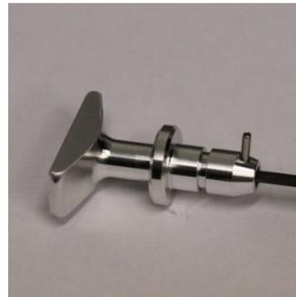
Slide the dipstick into the handle and line up the hole in the dipstick with the hole in the handle then place the new pin in place and tap it in with a hammer.
