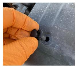
1. Remove the plastic pins holding the black plastic radiator cover and remove the cover.
