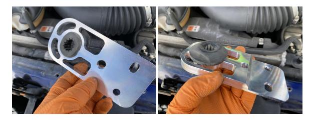
3. Insert the rubber grommets into the new billet aluminum radiator mounts.
