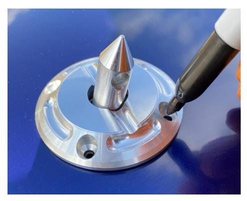
7. Apply the supplied adhesive rings to the bottoms of the bezels, but leave the lining in place so you can position the bezels on the hood to find the proper orientation. Center the bezels on the hood pins until they sit flush against the hood skin. Once you find the proper position for each bezel, mark the location of each of the [4] screw holes with a Sharpie marker or something similar.
