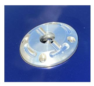
10. Remove the adhesive lining on the bezels and place them onto the hood, making sure to clock them properly and center them over the four pilot holes. Then use a phillips screwdriver to install the four screws. Do not over torque these screws! They only need to be snug.
