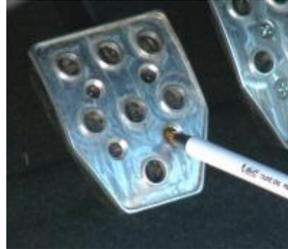
2. Using a 7/64 drill bit and drill, drill pilot holes for the screws in the marked locations. Repeat for each pedal.
