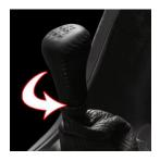
1. Remove the factory shifter knob by simply unscrewing it counter-clockwise.
