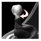
3. Install the new shift knob by simply screwing it on by turning it clockwise. Tighten the locking nut to secure the shift knob in place.
