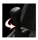
1. Remove the factory shift knob by simply unscrewing it counter-clockwise.
