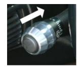
2. Using the supplied allen wrench, tighten the allen set screw to lock the Turn Signal Knob in place.
